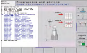
KinematicOpt & KinematicComp (Touch probe cycle for automatic measurement)
