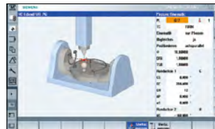
5-axis kinematic measuring cycles
