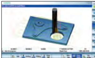
Simulation and machining contour monitoring
