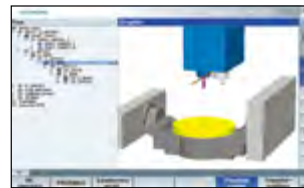
3D collision avoidance and collision avoidance ECO
