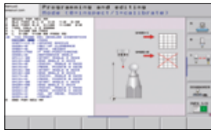
KinematicOpt & KinematicComp option (Touch probe cycle for automatic measurement)
